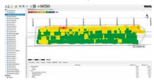
The primary purpose of Q Pave is to record temperatures. Aside from its core element, the pave navigator (a surface temperature sensor), the system makes it possible to manage various other temperature measurements and the screed extension.
